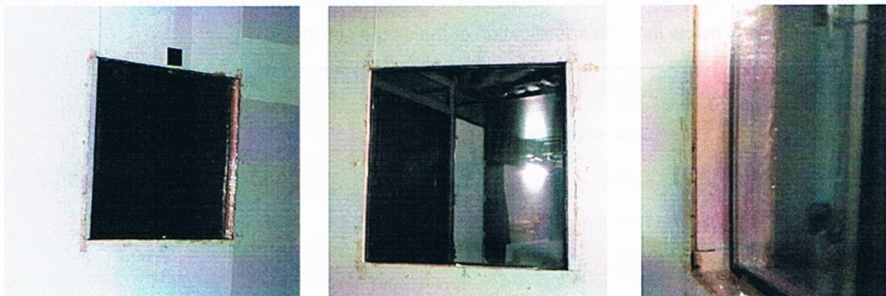
Figure 3. Photos of the installation. Left: view from outdoor side; middle: view from indoor side; right: zoom-in view of the gap between specimen and single glazing (the specimen is on the left)
